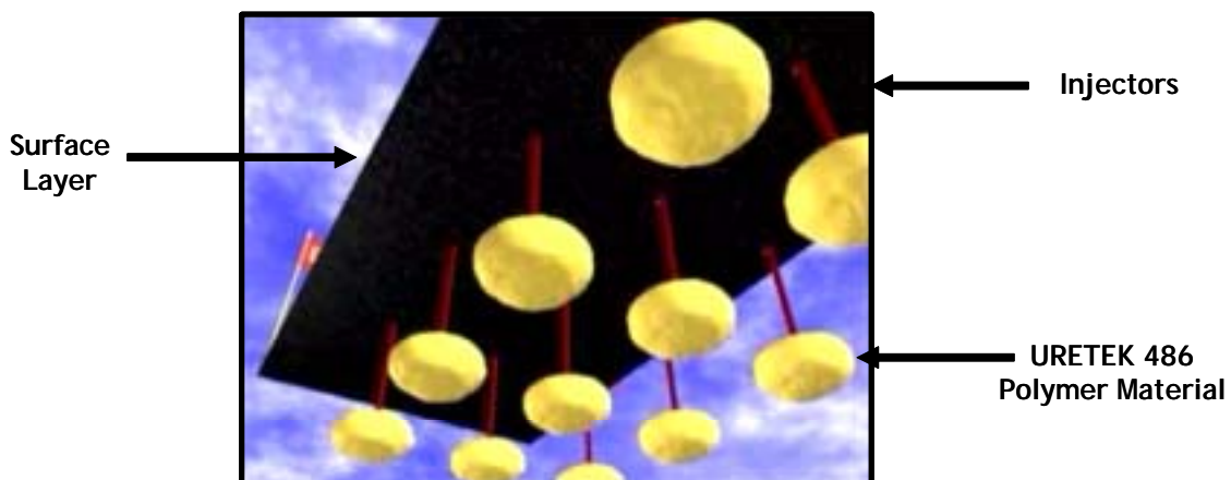
Figure 4: Injection Process using the Patented URETEK 486 Polymer Material
